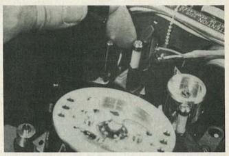
DURING PLAY OR RECORD operation, only motion applied to supply-reel turntable comes from tape being drawn out of cassette. Yet, turntable cannot be left free to "coast." Tape tension must be maintained so that tape stays in close contact with heads throughout transport.
