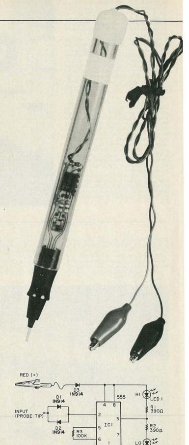
FIG. 1—SCHEMATIC DIAGRAM of the logic probe. Device can be powered by 3.5 to 15 volts tapped off the supply in the device under test.
