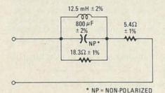
FIG. 3—IHF-STANDARDIZED load used for speaker simulation. Component values are critical.
