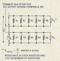
FIG. 1—SCHEMATIC illustrating principles of resistor-ladder construction.
