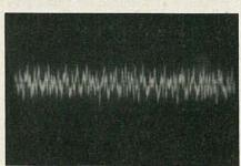
FIG. 7—NOISE IS REDUCED as compared to Fig. 6 when unmodulated groove is traced by new servo-controlled pick-up arm.
