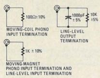
FIG. 4—SCHEMATIC DIAGRAM of the three common low-level input and output loads.
