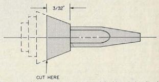
FIG. 6—THE PROBE TIP IS SALVAGED and adapted from the housing of a popular ballpoint pen.
