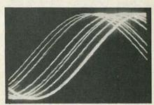
FIG. 3—SUBSONIC ARM RESONANCE distorts audible test tone.
