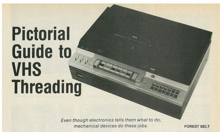
A VHS CASSETTE RECORDER THREADS tape into the transport only for the PLAY and RECORD modes. Pressing the STOP button causes the mechanism to unthread the tape and then return it to the cassette.
