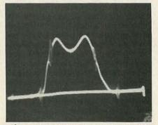
FIG. 6—ALIGNMENT IS COMPLETED. Dip in the center is normal in this receiver.
