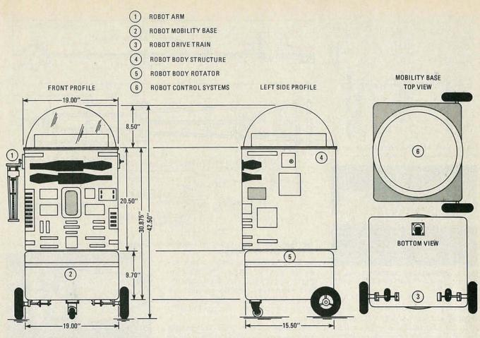
Fig. 1—DIMENSIONS of Unicorn-One as described in text. Size is not critical, though, and scale or dimensions may be altered to suit the requirements of the builder.
