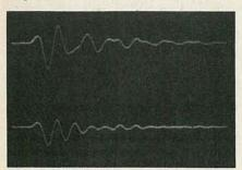
FIG. 5—EXTERNAL SHOCK applied to turntable cabinet is accented by arm resonance. Upper trace shows effect of external shock on conventional pick-up arm, while lower trace shows effect on servo-controlled arm.
