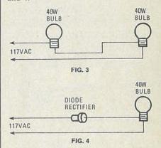
Don found that the measured voltage across all three bulbs was the same. He measured equal current in both circuits. You would expect the three bulbs to be of equal brightness but that was not so. The bulb brightness in one circuit was much greater than in the other.
