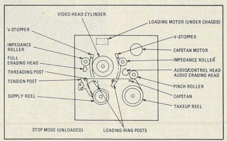
posts through complete arcs (about 110 degrees), both posts encounter V-shaped stop blocks. A loading-end switch signals loading-motor drive stage to stop motor. Similar signal activates pressure-roller solenoid, which draws roller against capstan.
