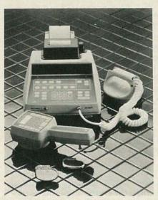
THE MEDTRONIC PACEMAKER programmer and two of the small Spectrax-SX pacemakers
