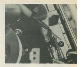
SIMPLE FAILURE of machine to load tape after PLAY button has latched down can point to broken or slipped drive belt. Characteristic of this symptom: slight whine of loading motor running but no hint of movement in threading mechanism. After several seconds without loading activity, automatic shutoff takes over and pops PLAY button back up.
