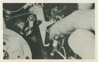
FAST FORWARD AND REWIND both operate only with tape unthreaded. Tape path carries it across front of cassette, with gate open, of course. Either operating button closes switch contacts that turn on capstan drive-motor. (Video-head cylinder, which has its own drive, remains off, in some machines.)
