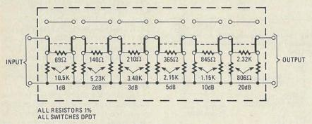
FIG. 7—STEP ATTENUATOR schematic. This device permits evaluation of output signals at predetermined input levels. DPDT switches may be either toggle or rocker type.
