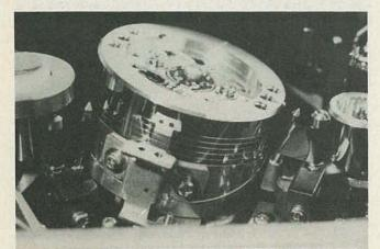
**TAPE POSITIONING** in transport can be critical. Guides and posts along path take care of that positioning. However, probably the most crucial are guide posts on loading rings (photo above). They align tape with respect to head wheel and thus with spinning video heads. Even slight misadjustment of just one guide post delivers band of snow (photo above, right). In some cases, you see multiple bands across picture. This symptom may not be too bad with tapes recorded on same machine.
