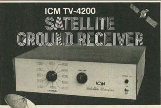
International incorporates advanced technology at its best in a fully packaged and assembled receiver covering all satellite channels 3.7-4.2 GHz band. Standard dual audio outputs provided at 6.2 and 6.8 MHz.
