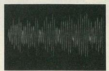
FIG. 6—NOISE WAVEFORM generated by unmodulated record groove that is traced with a conventional pick-up arm.
